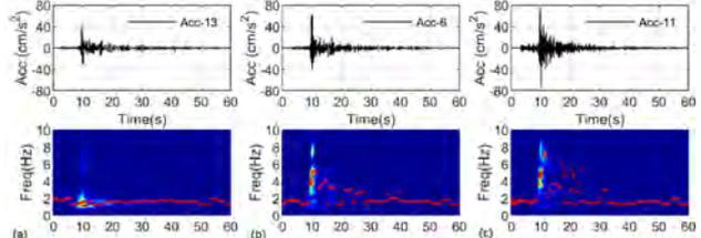
Fig. 5. CWT & IF results March 30, 2018 EQ. (a) girder (low frequency dominant), (b), (c) Piers (high frequency shift (4~6 Hz)).
