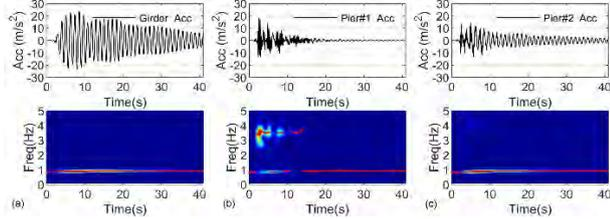
Fig.2.CWT time-frequency map and Instantaneous Frequency (IF) of acceleration responses from (a) continuous girder, (b) pier with movable bearing (c) pier with locked isolator bearing.
