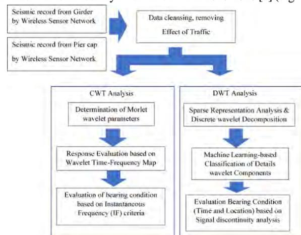
Fig.1. Methodology for Detection of bearing malfunction using CWT & DWT Analysis [1]
