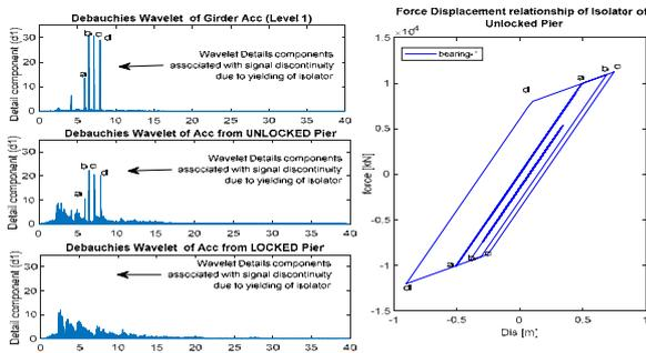
Fig.3. Example of simulation using discrete wavelet transform to detect the signal discontinuity associated with yielding of bilinear isolator system.
